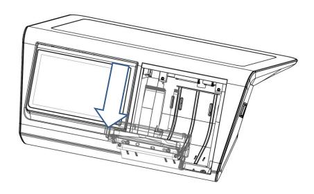
Step 7 Connect the FPCs of the new printer module onto the PCB.
