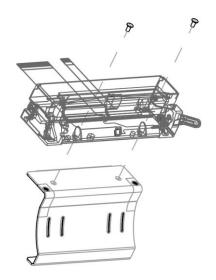
Step 6 Disconnect the two FPCs from the PCB.
