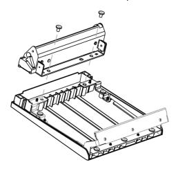
Step 11 Fix the printer door back onto RiPac-10P1 and close up the door.
