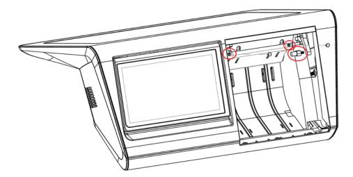
Step 5 Unscrew two screws on the printer assembly to take down the printer module.
