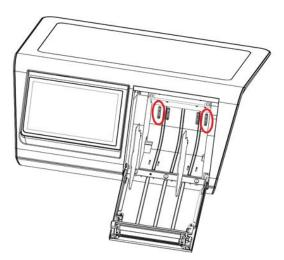
Load the paper roll in between the two holders then close the printer door.
