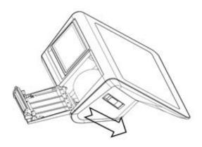
Step 2 Unscrew the three screws that connects the printer doo to the device in order to take down the printer door.
